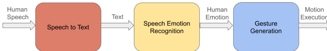
Fig. 3. The human speech emotion recognition to robot gesture mapping pipeline
