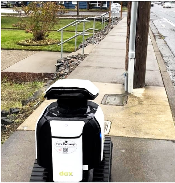
Fig. 14: DAX attempting to navigate around an awkwardly placed lamp post. Please note the vertical falloff on the left.
