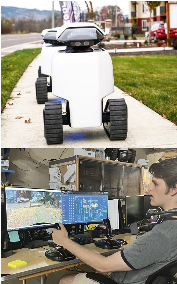
Fig. 2: The DAXBot software, interfaces, and hardware. Each new deployment location has a custom base station to support communications, including realtime video, audio, GPS, robot status and connectivity. During the robot driver observation period, DAXBot, with an operations team of 5 people (includes driving and maintenance) and 26 robots, was just beginning to test autonomous navigation features after two years of active human-in-the-loop delivery.
