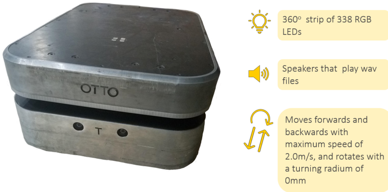
Fig. 2. The OTTO 100 and channels of communication
