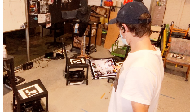
Fig. 1: This paper presents an experimental study and the resulting technology improvements based on participants’ ratings and perspectives. The figure features the robotics chairs and the mobile teleoperation UI for controlling them.
