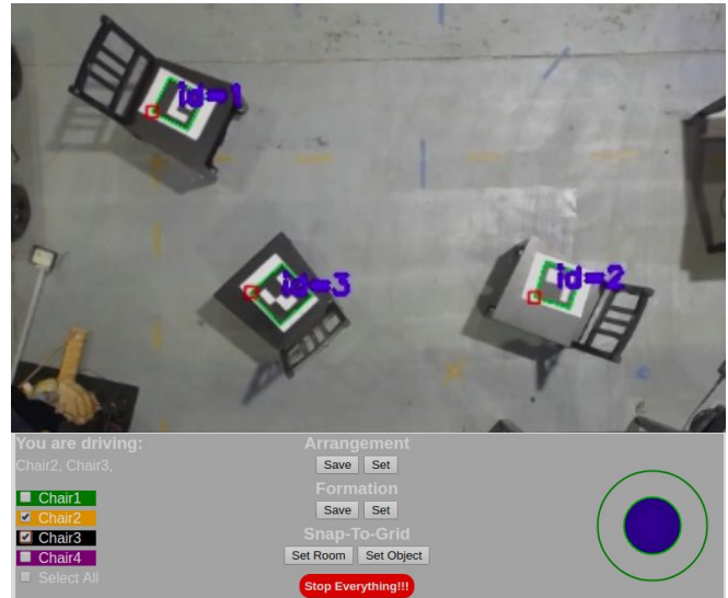
Fig. 5: Screenshot of the added screen-based user interface on being run on a personal computer.
