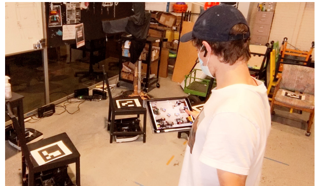
Figure 1: A user interacts with the Tele-ChairBots interface on their mobile tablet to control multiple ChairBots.
