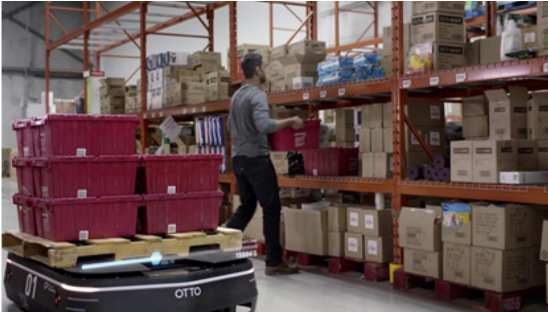
Fig. 1. At factories and warehouses, the OTTOs work closely with people and other automated technologies as they load up the OTTOs at one location and then the OTTOs travel to another location, where people or automated life unload them.
